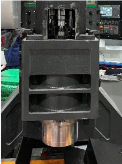
Imported high-speed direct drive spindle
