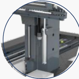
Lifting part of the moving beam
